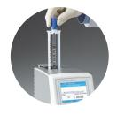
Insert assay tube into the cobas® Liat® Analyzer.
